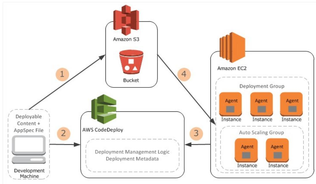
Figure 6: AWS CodeDeploy process
